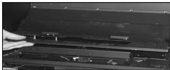
Figure 48: Burner Tray Installation.
